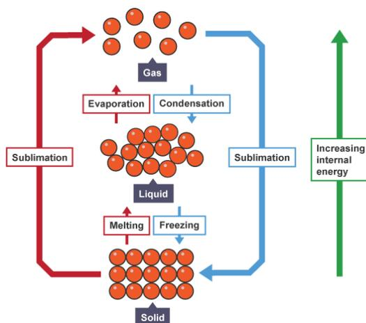
Mass is conserved when a substance changes state. If you start with 1kg of oxygen gas and cool it, you will have 1kg of liquid oxygen.
