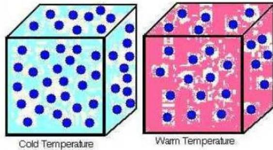
Different states of a material have different densities because of particle arrangement:
